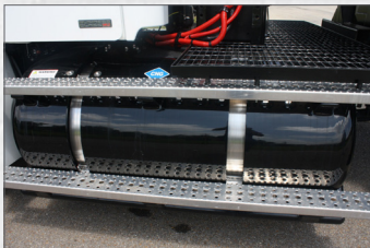
▲ Pac-Mac can accommodate a variety of CNG tank options including below the rail saddle tanks or back of cab, above rail tanks
